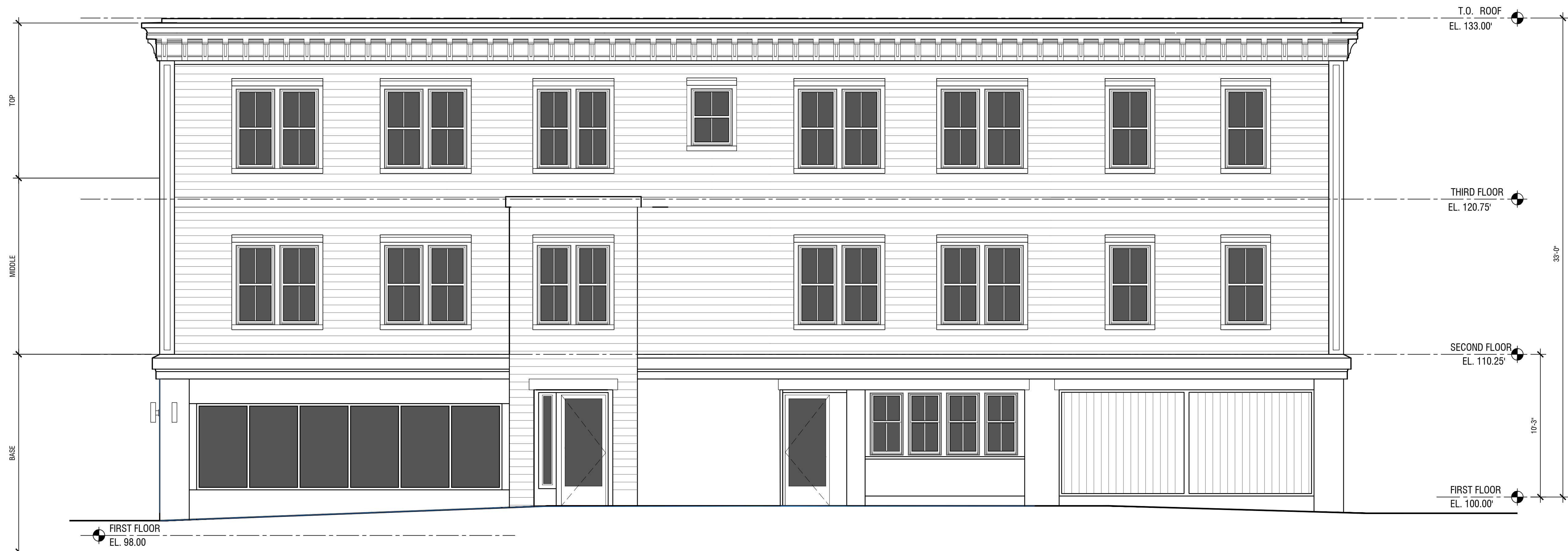
2 WEST ELEVATION - SOUTH STREET SCALE: 1/4" = 1'-0"
