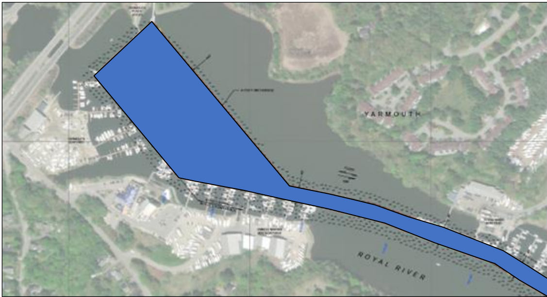
Figure 16: Royal River Federal Navigation Project. (The blue shading represents the current design of the FNP and anchorage.)
