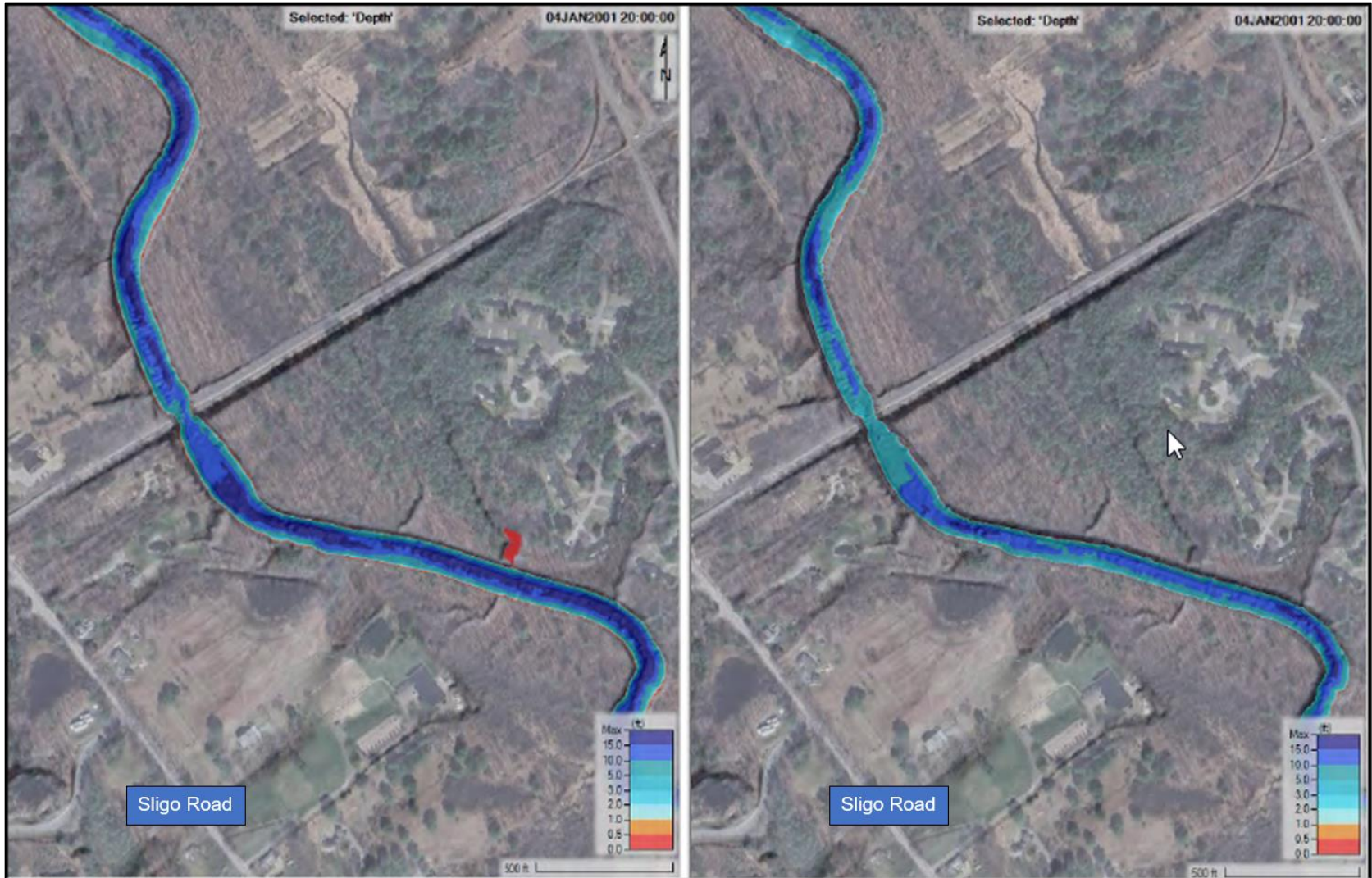
Figure 36: Comparison of Existing (left) and Projected (right) River Depths at Annual Median Flows Upstream of the East Elm Street Dam, Near the Maine Central Railroad Bridge
