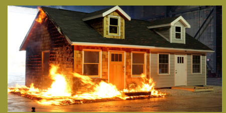
Figure 1 – Creating and maintaining home ignition zones (defensible space) around your property are proven ways to reduce risks of property damage during a wildfire, as tests at the IBHS Research Center have shown.
