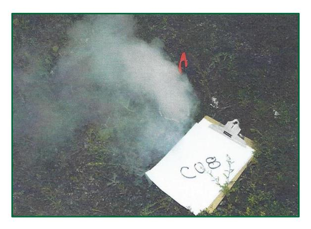
Smoke coming out of ground at clean out. Pipe is obviously broken and not capped.
