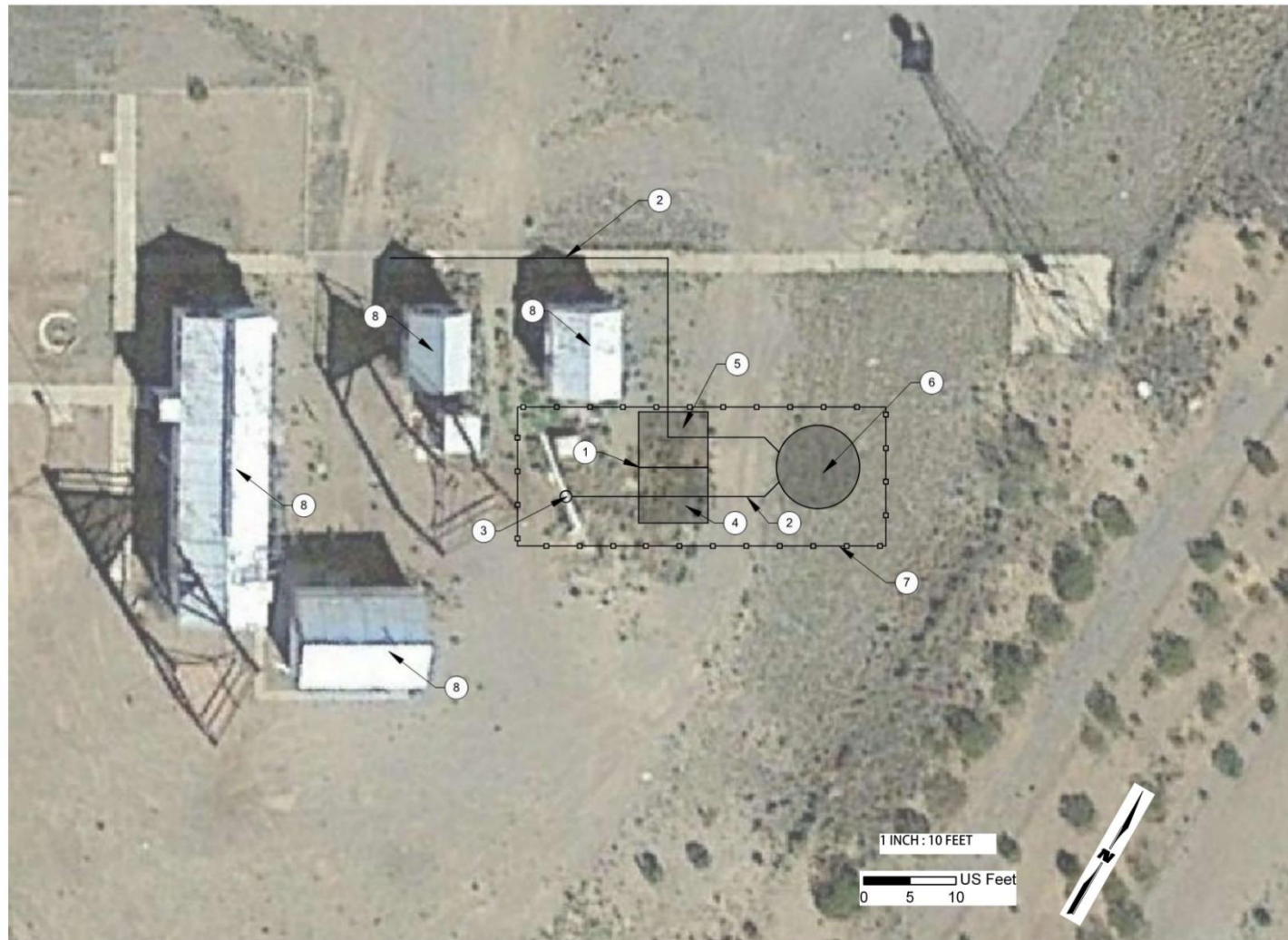
Figure 22: Airport Alternative X New Ground Water Storage Tank without Fire Flow
