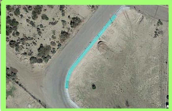
Figure 106: Detail of recommended sidewalk at northeast corner of N. Pershing St. and New School Rd.
