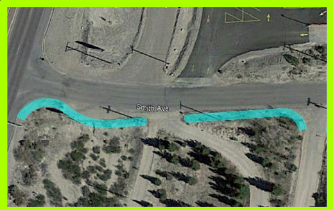
Figure 76: Detail of recommended sidewalk, southeast corner of N. Date St. and Smith Ave.
