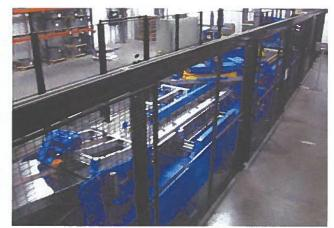
Soenen Core Cutting machine in VTCR
