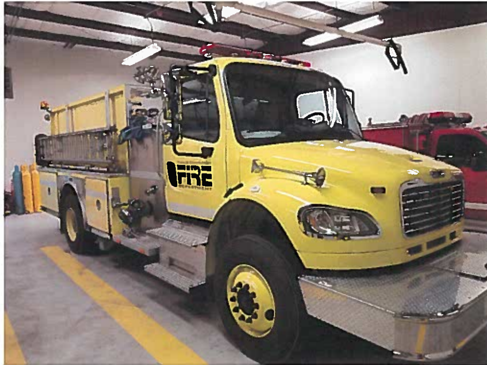
2013 – New E-One Engine Truck 1000 Gallons water 1250 GPM Pump
