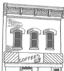
INAPPROPRIATE DESIGN: Do not infill the transom with brick or wood, or cover it over with signs.
