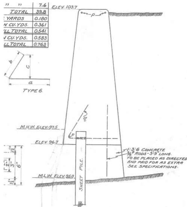
Figure 7: Wall detail from 1926 Plans for Concrete Seawall
