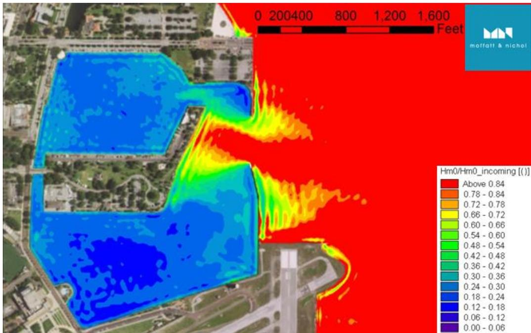
Figure 15 H<sub>s</sub> reduction factor ( $T_p=7\text{sec}$ ,  $\theta=120^\circ$ )
