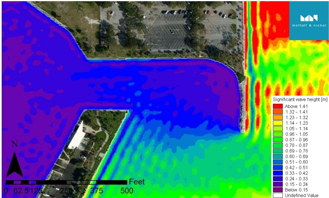
Figure 21 Maximum wave height at the location of the transient docks for the 100-year storm event
