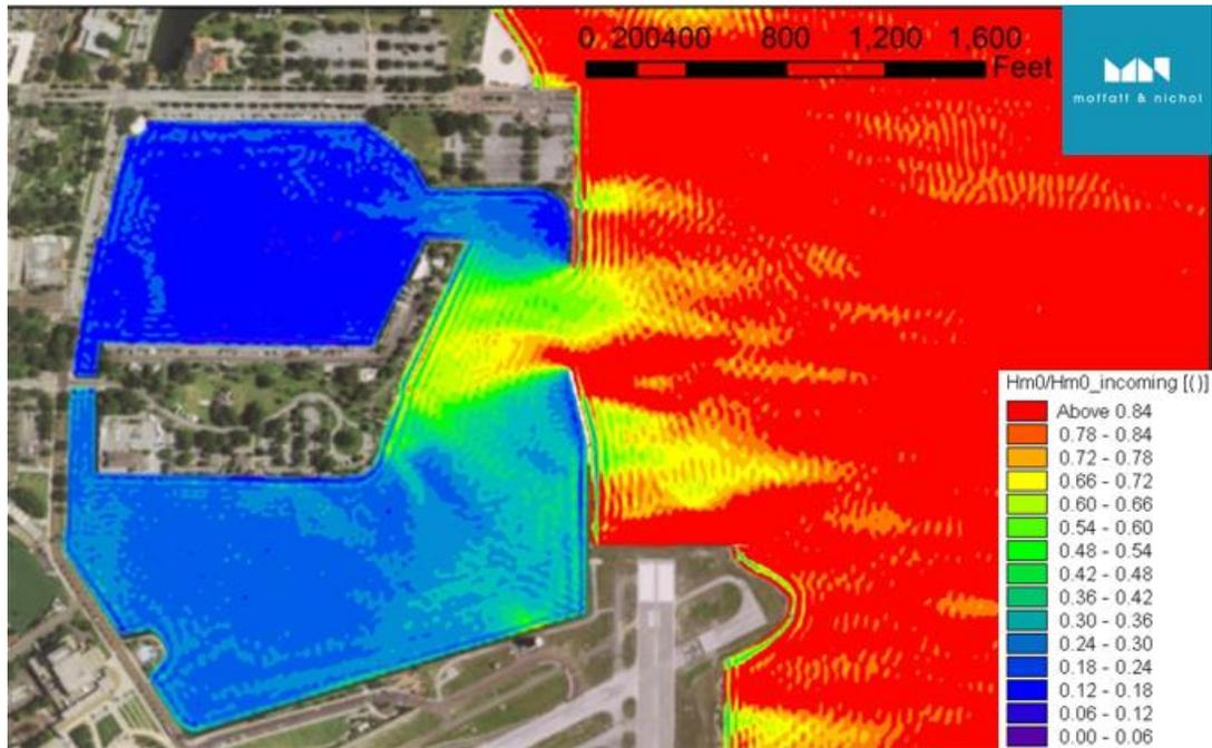
Figure 8 H<sub>s</sub> reduction factor ( $T_p=4\text{sec}$ ,  $\theta=90^\circ$ )
