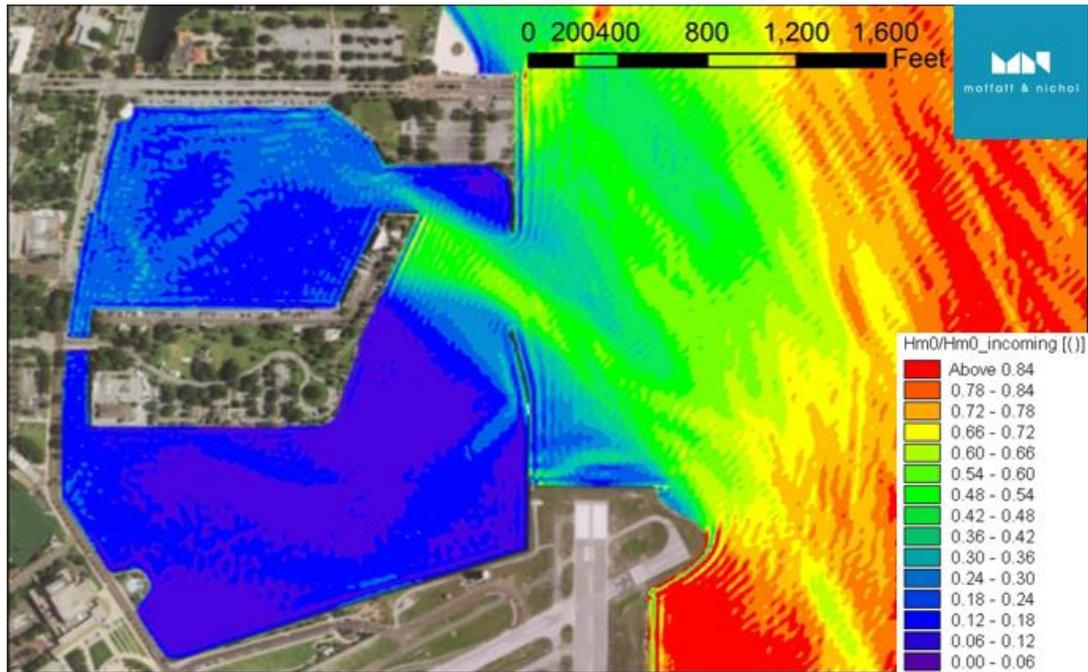
Figure 12  $H_s$  reduction factor ( $T_p=4\text{sec}$ ,  $\theta=150^\circ$ )
