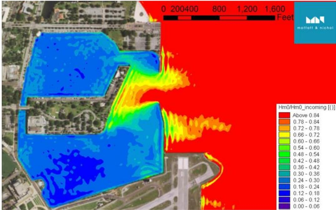
Figure 14 H<sub>s</sub> reduction factor ( $T_p=7\text{sec}$ ,  $\theta=105^\circ$ )
