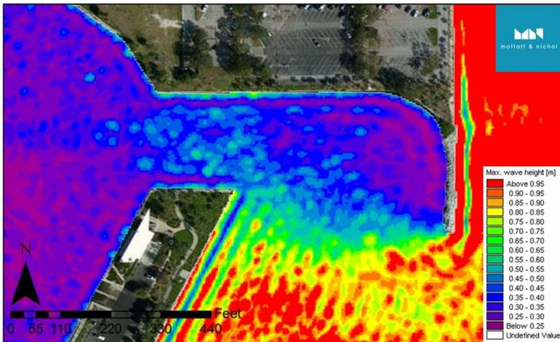
Figure 18 Maximum wave height at the location of the transient docks ( $T_p=4\text{sec}$ ,  $\theta=90^\circ$ )
