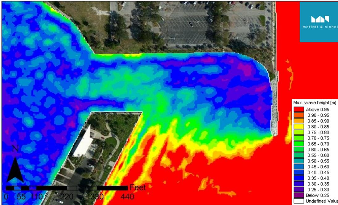
Figure 19 Maximum wave height at the location of the transient docks ( $T_p=7\text{sec. } \theta=90^\circ$ )
