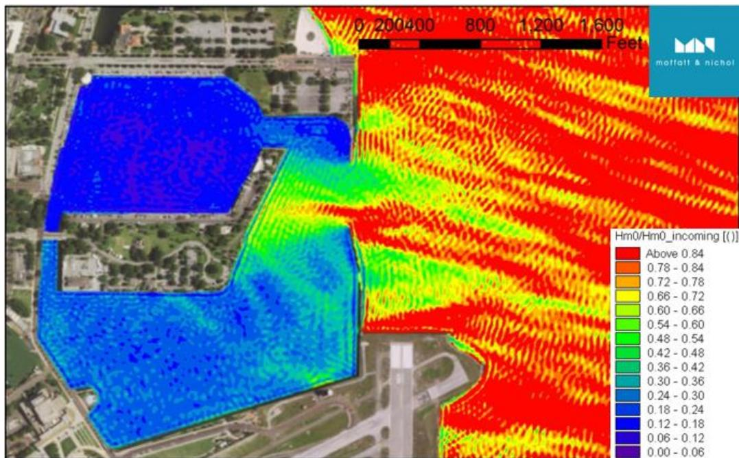
Figure 9 H<sub>s</sub> reduction factor ( $T_p=4\text{sec}$ ,  $\theta=105^\circ$ )
