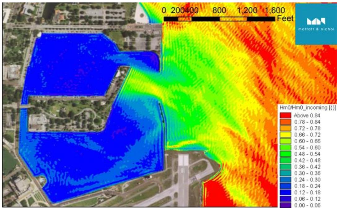
Figure 11  $H_s$  reduction factor ( $T_p=4\text{sec}$ ,  $\theta=135^\circ$ )
