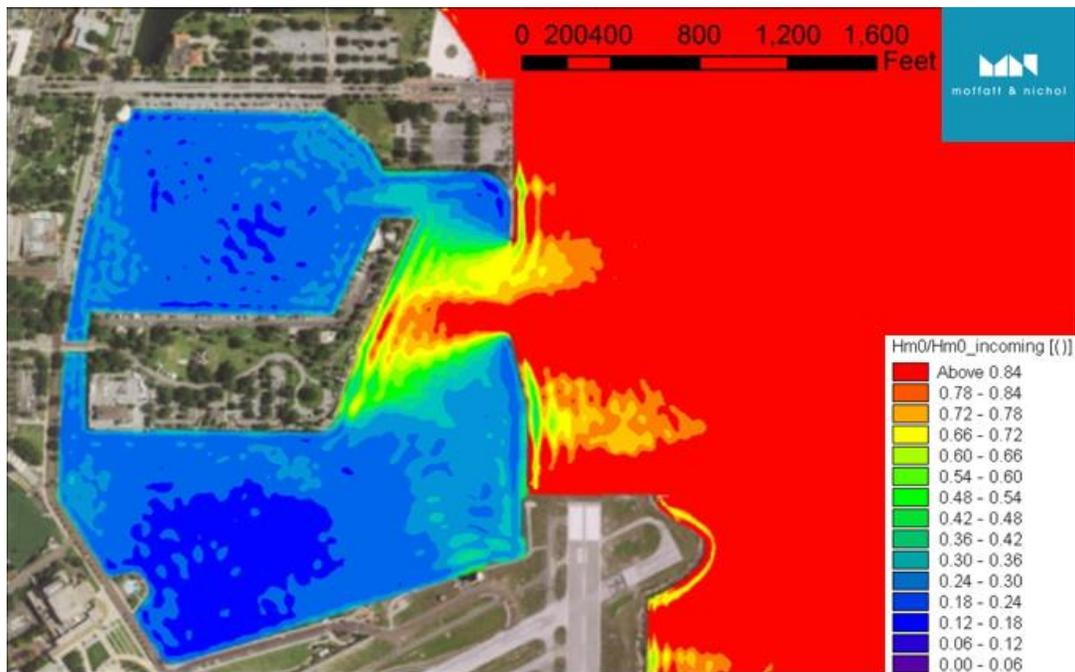
Figure 13  $H_s$  reduction factor ( $T_p=7\text{sec}$ ,  $\theta=90^\circ$ )
