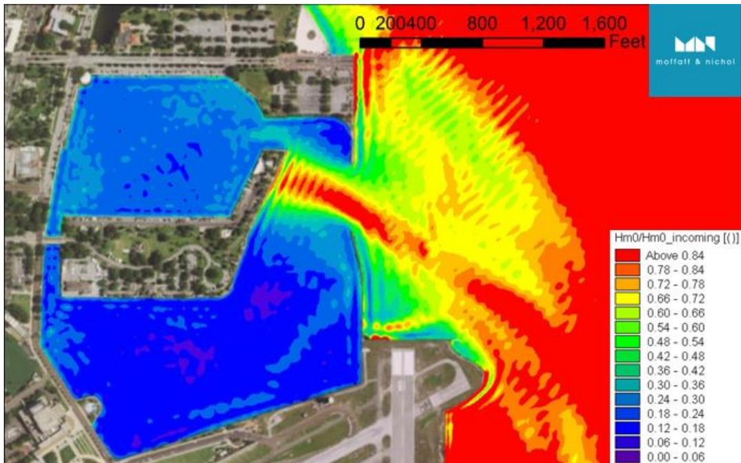
Figure 17  $H_s$  reduction factor ( $T_p=7\text{sec}$ ,  $\theta=150^\circ$ )
