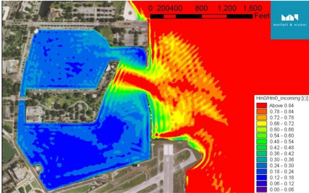
Figure 16  $H_s$  reduction factor ( $T_p=7\text{sec}$ ,  $\theta=135^\circ$ )
