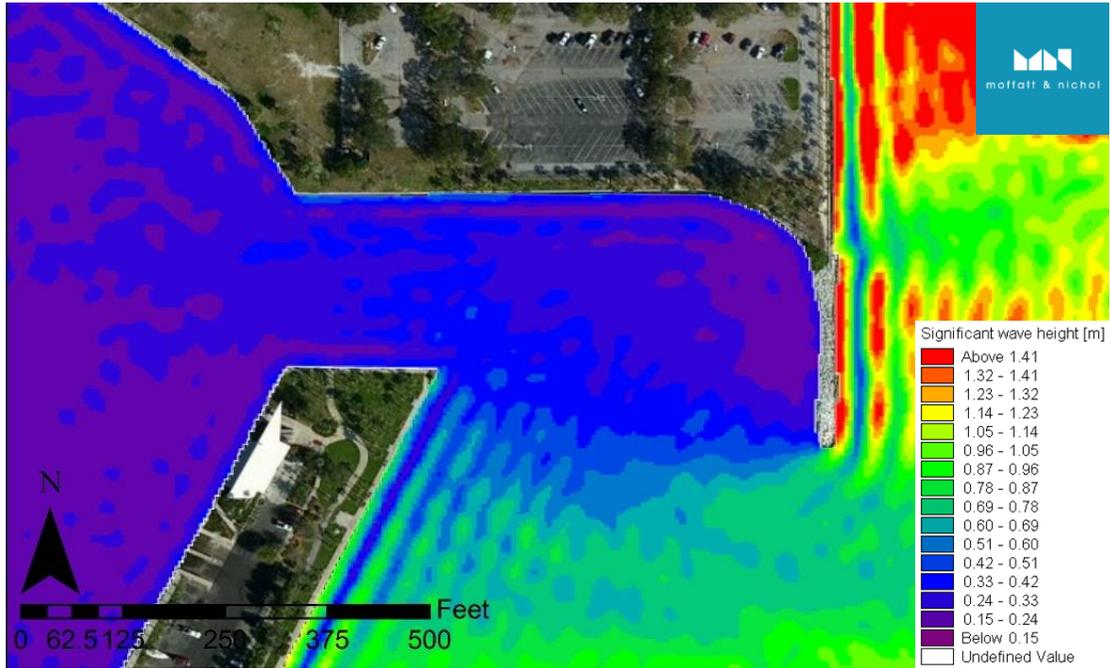
Figure 20 Maximum wave height at the location of the transient docks for the 50-year storm event
