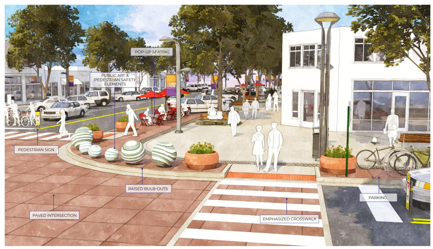
FIGURE 4-12: CENTRAL AVENUE INTERSECTION WITH RAISED BULB-OUTS - LONG TERM ENHANCEMENT
