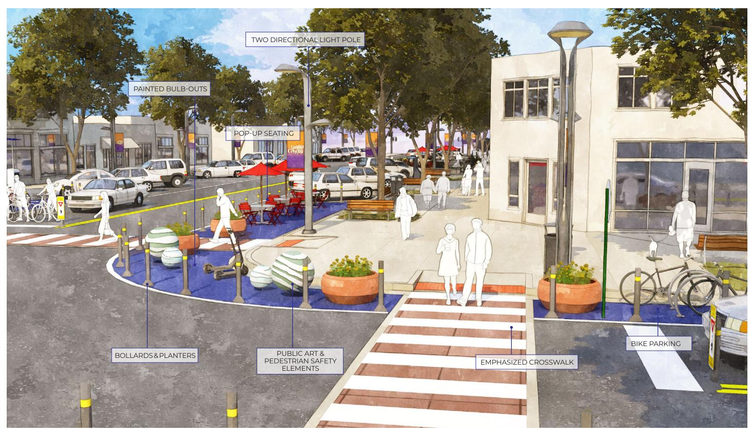
FIGURE 4-11: CENTRAL AVENUE INTERSECTION WITH PAINTED BULB-OUTS - SHORT TERM ENHANCEMENT
