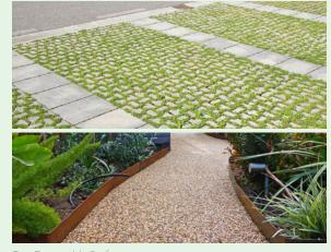
Top: Permeable Surface Bottom: Permeable Walkway
