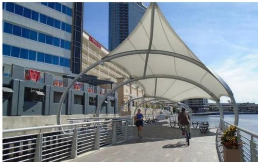
The covers should be high tension fabric similar to the system used at the Tampa Riverwalk (see image). The design should be sufficient to withstand hurricane force winds.
