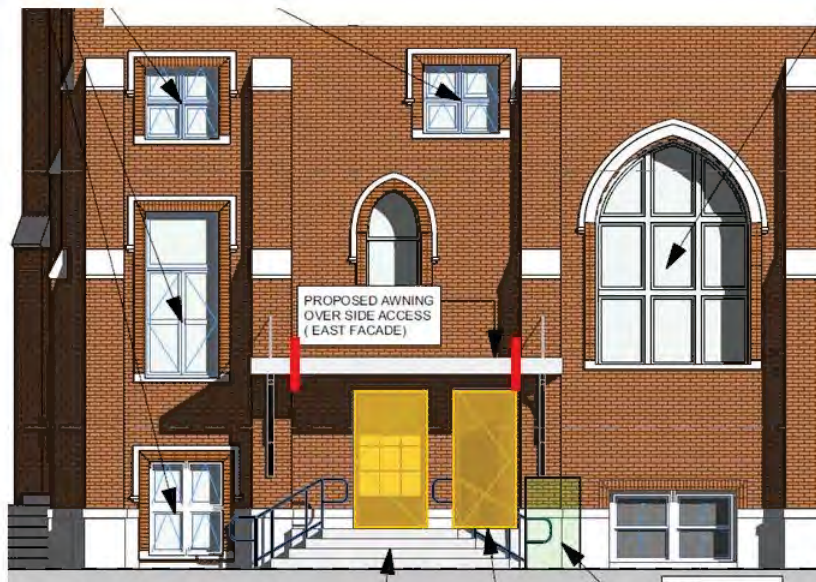
Figure 2: Proposal with the awning that obscures the buttresses and two new door openings.
