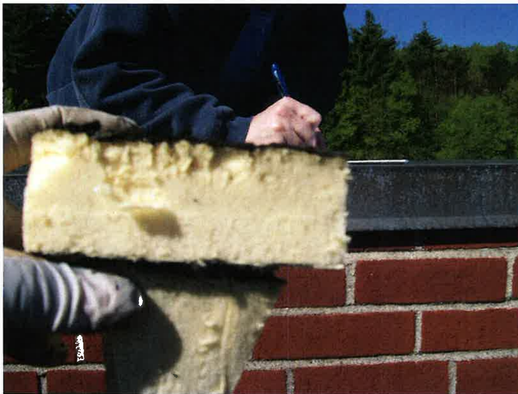
Layer of "Poly Iso" from 1991 High Roof
