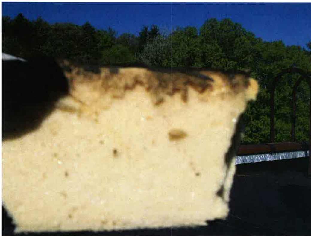
Layer of "Poly Iso" from gym roof
