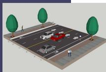
Elements like pedestrian refuge medians within the roadway, pedestrian-activated traffic signals or flashers, pavement striping and signage can be used to improve safety and comfort for all users.
