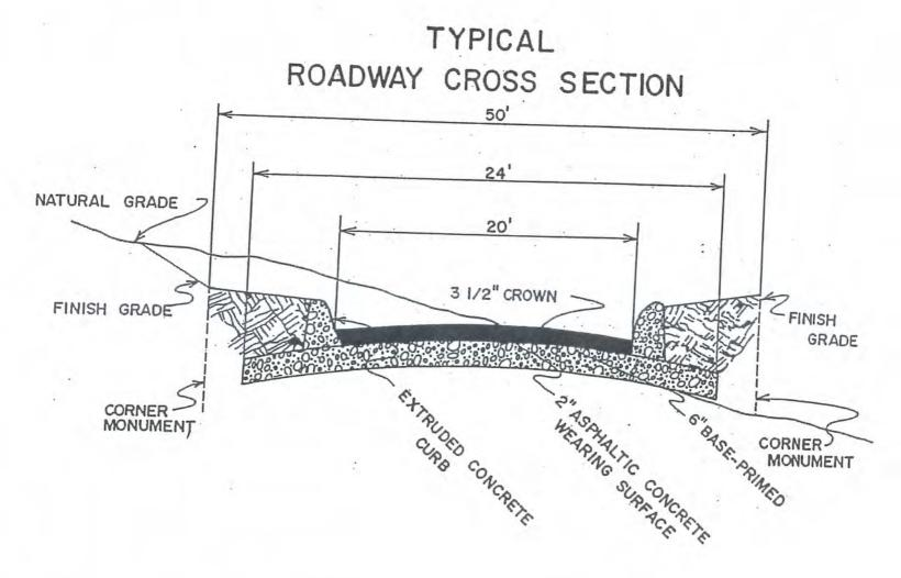
Note: Curbs are not required. A two foot compacted shoulder is required if curbs are not used.
