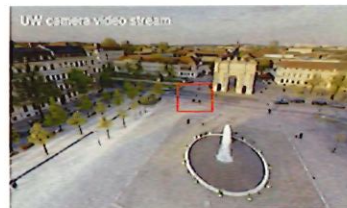
Improved situational awareness with ultra wide (90 deg) FOV view with frame indicating zoomed in area
