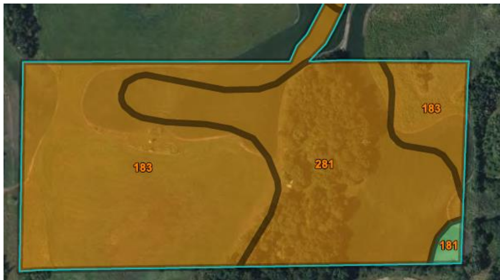
Soil Types Delineation #181 Litchfield loamy sand 1%; #183 Forada sandy loam 56%; # 281 Danfur coarse sandy loam 43%
