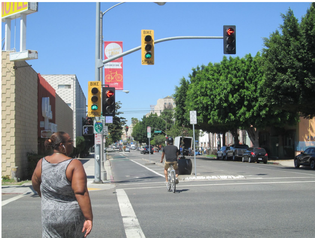
A Class IV bikeway buffers cyclists from traffic and door zones of parked cars.
