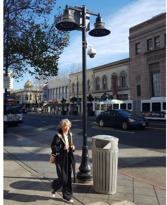
In addition to standalone pedestrian-scale lighting, street lights can be fitted to include pedestrian-scale fixtures that illuminate the walking area, while higher, vehicle-scale street lights illuminate the roadway.
