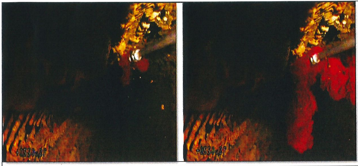
Figure 3: BESST uses a patented sideways injection down hole during the flow survey, which greatly increases the accuracy of the velocity measurements and the flow and mass balance calculations.
