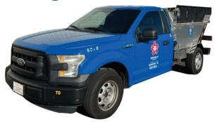
In Rolling Hills, we provide "scooter service" for all residents. Our drivers go onto the property to empty waste containers by hand into a "scooter truck," a small pickup truck with a special collection container in its bed. When full, the scooter truck returns to the large collection truck and offloads there.
