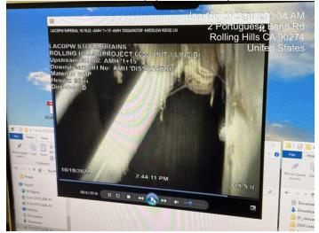
Photo 6 - Video clips were reviewed to determine length of corroded CMP from station to station.
