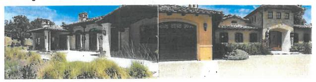
FIGURE 12 EXAMPLES ON LOT XXX OF GOOD LANDSCAPING CHOICES OF LOW FUEL VOLUME AND ADEQUATE SPACING BETWEEN PLANTS ALONG WITH HARDSCAPING TO PREVENT IGNITION FROM EMBERS
