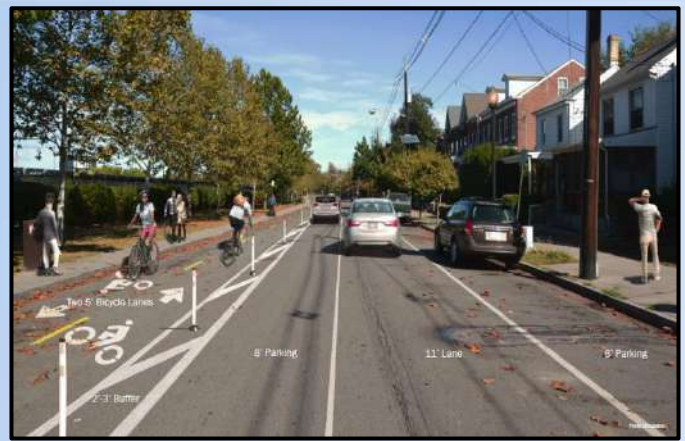
Above: Photo simulation of potential two-way cycle track on Lamberton Street in the City of Trenton. Source: NV5/ D&R Greenway Land Trust
