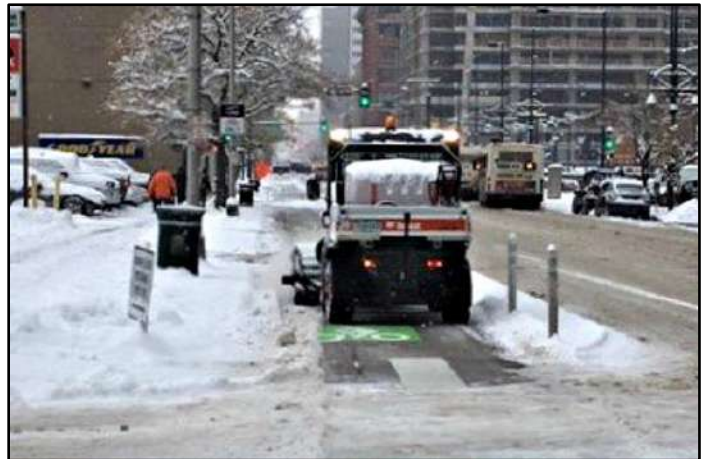
Above: Smaller snow plows such as the one above in Denver would need to be purchased and operated to clean and clear protected bicycle facilities of debris and snow.
