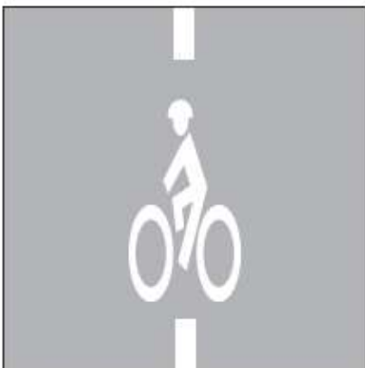
Bike detector pavement marking MUTCD Fig. 9C-7
