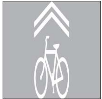
Shared lane marking MUTCD Fig. 9C-9
