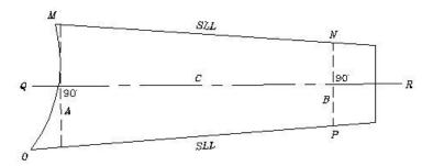
AVERAGE LOT WIDTH IS  $\frac{A+B}{2}$  AND LINE QR BISECTS ANGLE FORMED BY LINES MN AND OP EXTENDED. C IS THE PERPENDICULAR DISTANCE BETWEEN LINES A AND B, LINE NP MAY COINCIDE WITH LOT LINE.
