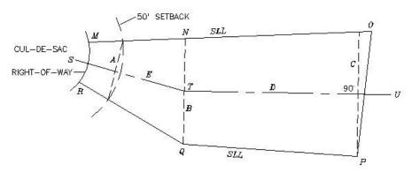
AVERAGE LOT WIDTH IS  $\frac{A+B}{2} imes \frac{E}{E+D} + \frac{B+C}{2} imes \frac{D}{E+D}$ , Line ST bisects angle formed by Lines MN and QR extended and line TU bisects angle formed by Lines NO and PQ extended. D is the distance between B and C. E is the distance between A and B.
