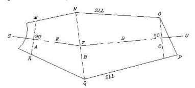
AVERAGE LOT WIDTH IS  $\frac{A+B}{2} imes \frac{E}{E+D} + \frac{B+C}{2} imes \frac{D}{E+D}$ , line ST bisects angle formed by lines NO and NO extended. NO is the distance between NO and NO extended. NO is the distance between NO and NO extended. NO is the distance between NO and NO extended. NO is the distance between NO and NO extended. NO is the distance between NO and NO extended NO is the distance between NO and NO extended and NO extended in the distance position of NO extended in the po
