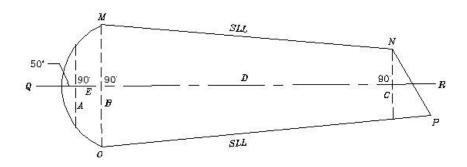
AVERAGE LOT WIDTH IS  $\frac{A+B}{2} \times \frac{E}{E+D} + \frac{B+C}{2} \times \frac{D}{E+D}$  AND LINE QR BISECTS ANGLE FORMED BY LINES MN AND OP EXTENDED. D IS THE PERPENDICULAR DISTANCE BETWEEN LINES A AND A
