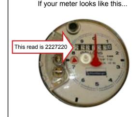
Write down the digits on the face of the meter starting from left to right. Include all the zeros <u>and</u> the stationary digit at the end which is painted on. *In total there should be seven (7) digits.*
