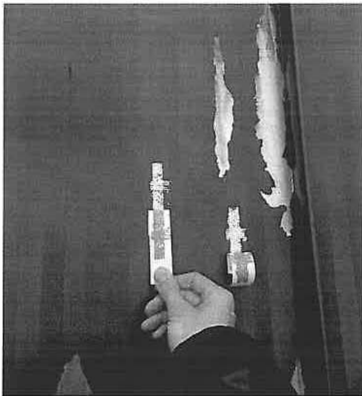
Photograph 9 – Test locations 2 (right) and 3 (left). Both OB with 90-100% of coating removed
