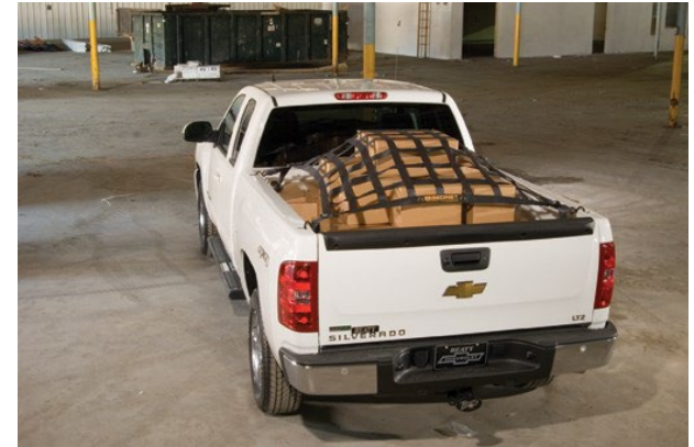
Properly secured loads utilize "bed nets" like this, tarps, and adjustable or ratcheting tie downs.
