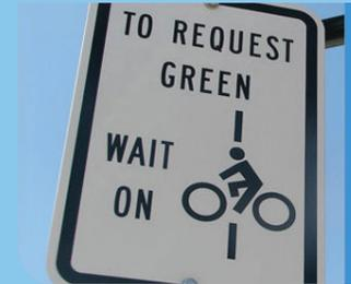
Traffic signals can use **bicycle detection** to cause the signal to turn green when a bicyclist is waiting at the stop line. This can be done automatically or the bicyclist can use a push-button. When automatic detection is implemented, striping should indicate where the bicyclist needs to stop to trigger the detector.
