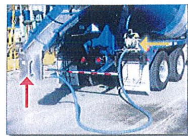
Figure 8. Chute washout bucket and pump
