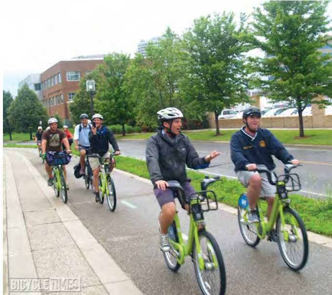
Separated- vertically and horizontally between road and track Pavement delineation- between walking lane and cycle lane Walking lane on building side to access homes and shops Cycle lane on road side to access intersections
