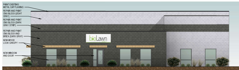
4 EXISTING BUILDING OFFICE AND WAREHOUSE - SOUTH 1/8" = 1'-0"
