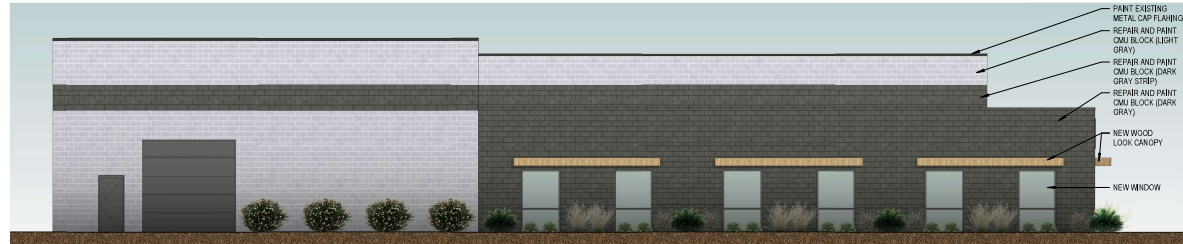
5 EXISTING BUILDING OFFICE AND WAREHOUSE - WEST 1/8" = 1'-0"
