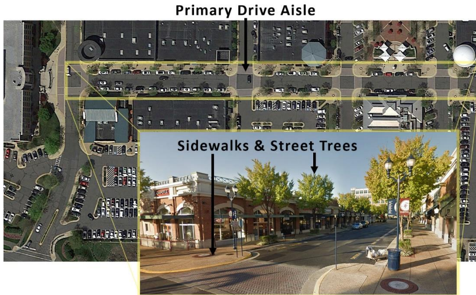
Figure 5-5: Design of Primary Drive Aisle
