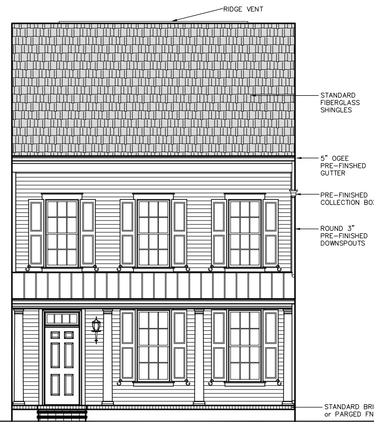
S2 FRONT ELEVATION SCALE 1/8" = 1'
