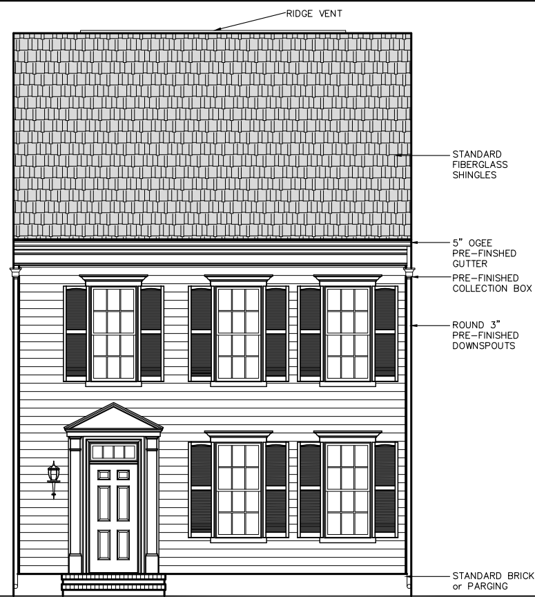
S3 FRONT ELEVATION GEORGIAN SCALE 1/8" = 1'
