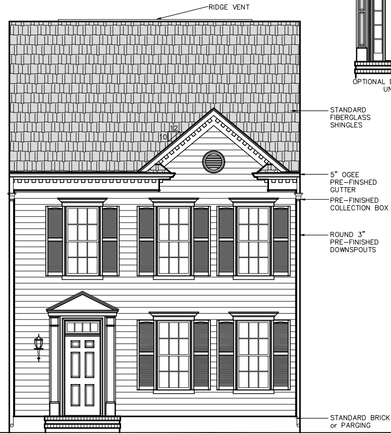
S3 FRONT ELEVATION GEORGIAN w/GABLE SCALE 1/8" = 1'
