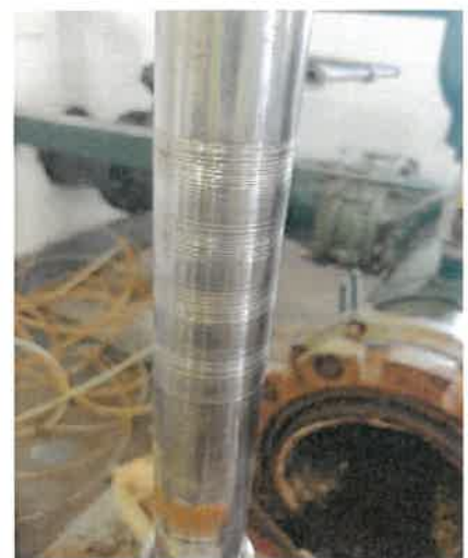
Removing the pump and motor at Palmer Springs and the scored pump shaft.
