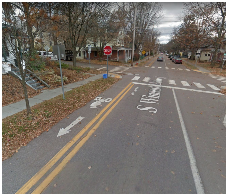
S. Winooski Ave, Burlington. Note the opposite-direction bike lane to the left of the double-yellow line. Screenshot from Google Street View.
