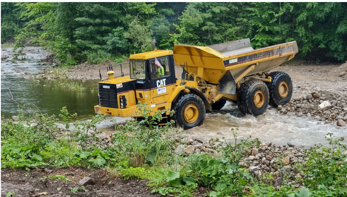
Figure 2: Haul unit crossing (reversing) at ford, discharge at crossing limited to fines washing off of tires that quickly dissipates before reaching end of work area.
