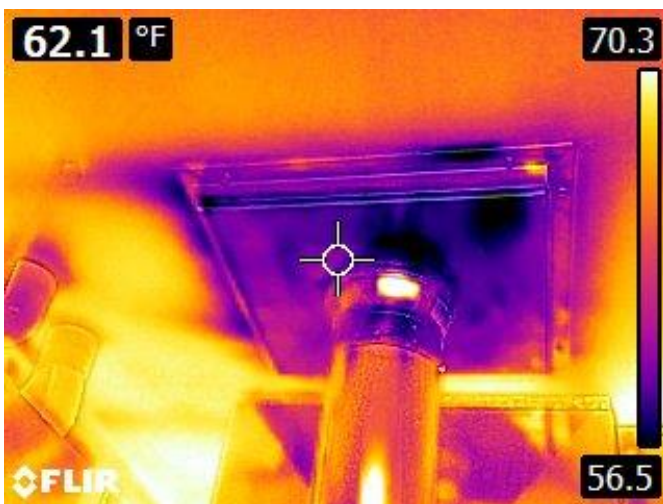
Air leakage around the exhaust flue pipe and around the perimeter of the metal pan.
