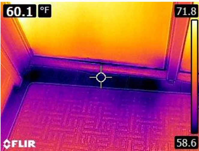
Air leakage at the threshold of the double doors on the south wall. Similar results were found at the double doors on the north wall.
