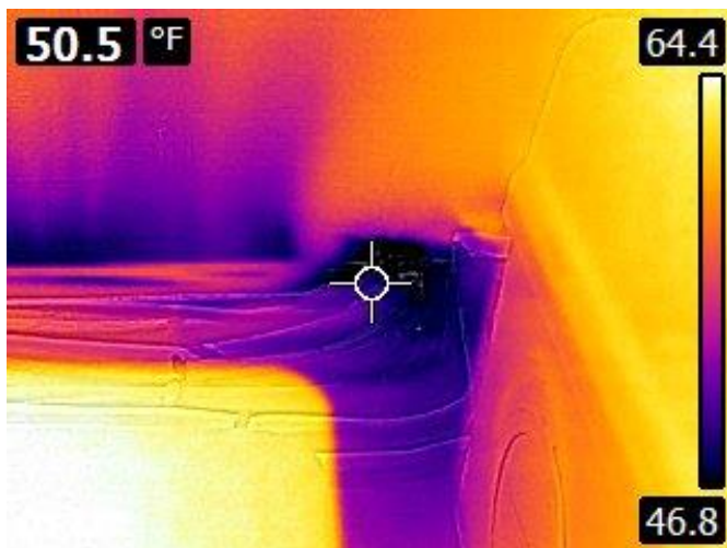
Air leakage through a hole made for wiring in the drywall ceiling of the boiler room and through the wall to ceiling connection.
