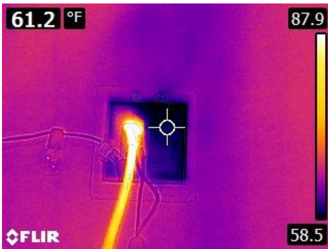
Air leakage through an electrical outlet on the south exterior wall of the open space room.
