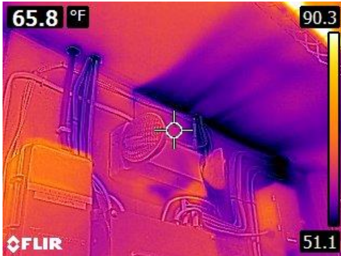
Air leakage through the wall to ceiling connection on the north wall of the boiler room and through holes in the drywall ceiling where wiring is being fed through.
