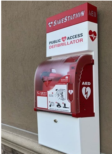
Example of an Automatic Electronic Defibrillator (AED) smart cabinet.
