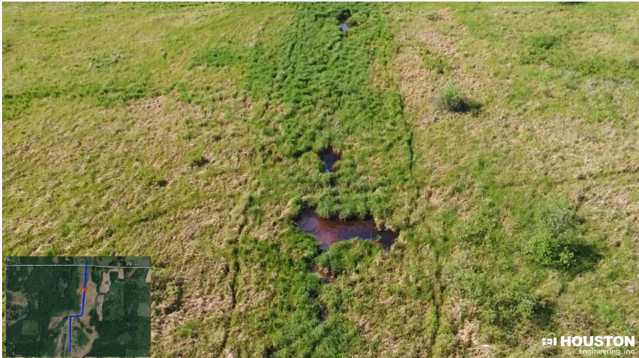
Photo 3: Poor channel definition at the upstream end of the Main Trunk and pooling, stagnant water.
