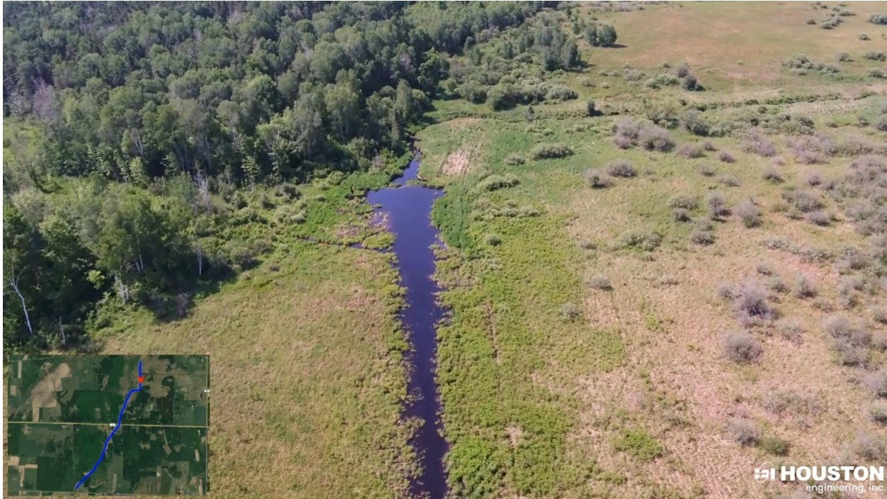
Photo 1: Obstruction at Main Trunk Station 253+00 that is causing water to pool upstream.
