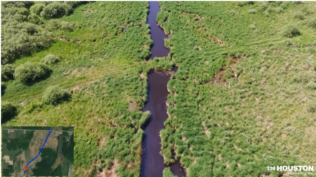
Photo 2: Field crossing at Main Trunk STA 100+00 that is in disrepair and obstructing flow.
