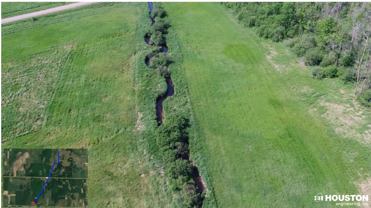
Photo 4: Meandering of ditch at Main Trunk STA 150+00 with trees growing in channel.
