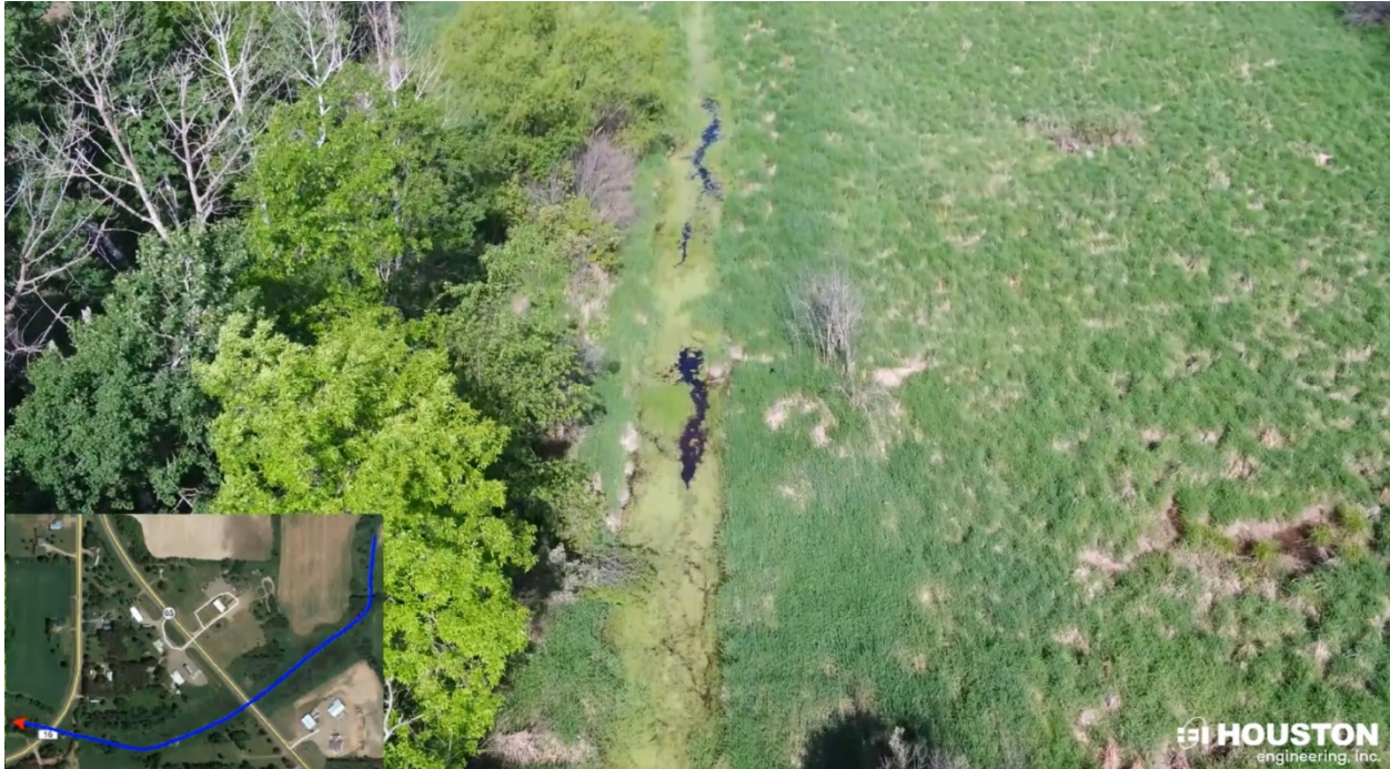
Photo 1: Algae growth in the ditch channel at Main Trunk STA 58+00.
