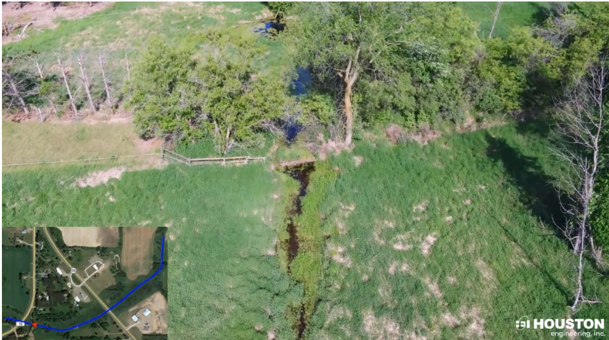
Photo 5: Flow blockage on Main Trunk caused by debris at STA 55+00.
