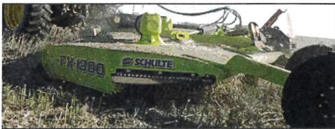
Outboard blade rotation keeps material from balling up under the deck
