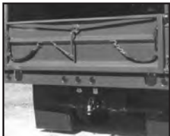
Eccentric lever top pin release
