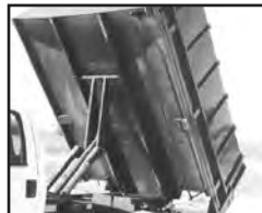
Low profile crossmemberless under-structure
