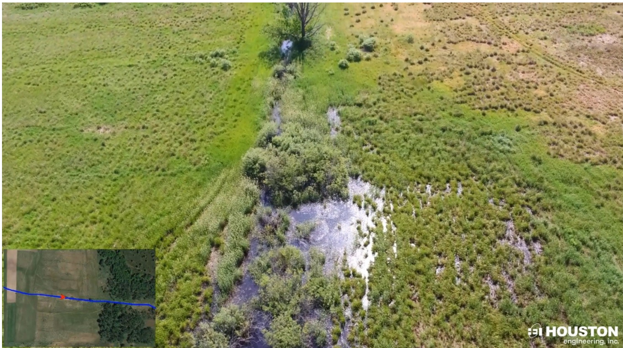
Photo 6: Poor channel definition at upstream end of Branch 1 with pooling, stagnant water.
