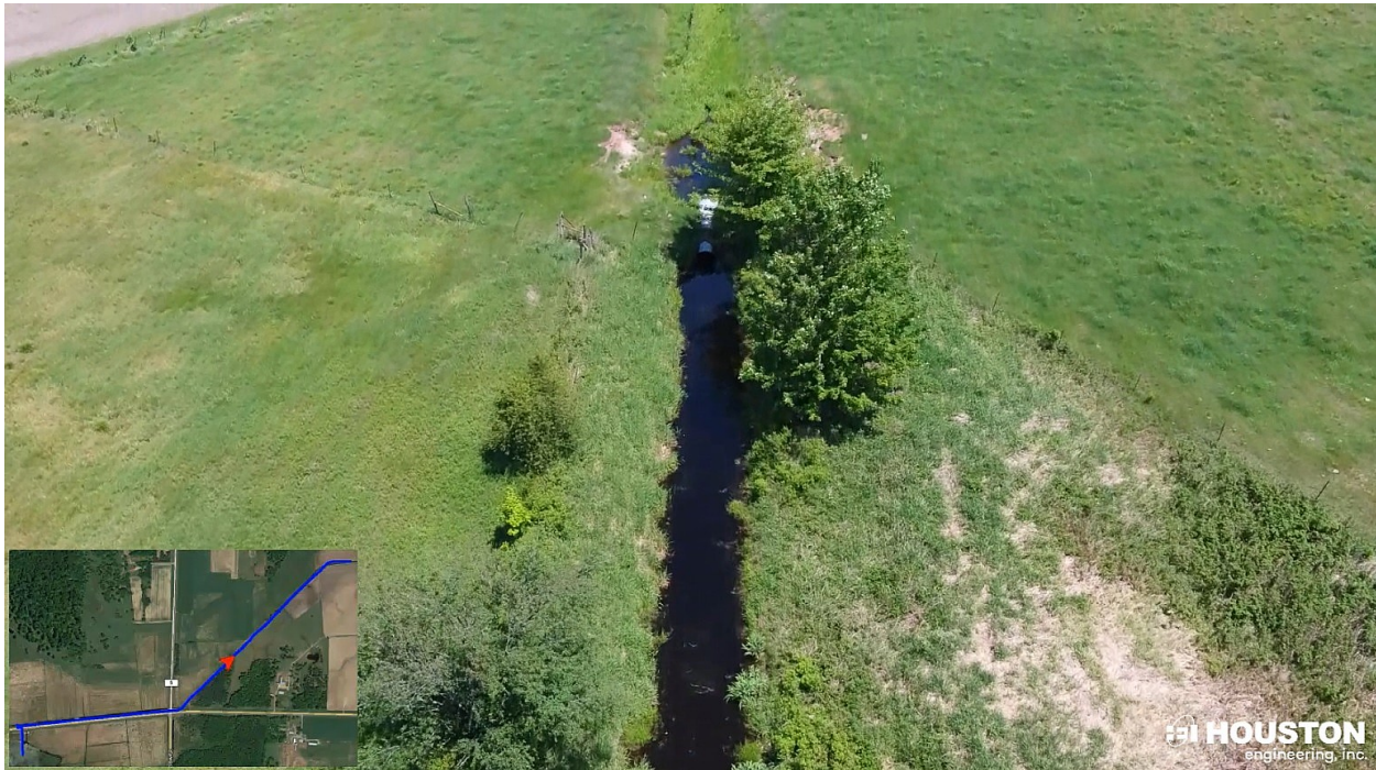
Photo 11: Branch 3 field crossing at STA 101+00 that is causing water to pool upstream.
