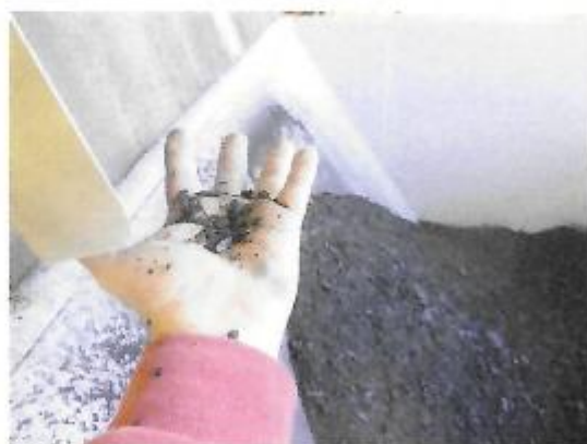
Solids generated by the Volute Dewatering Press.
