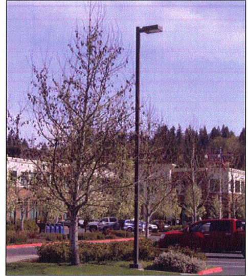
Cut-off lighting fixtures illuminate pedestrian and vehicular circulation areas while minimizing uplighting and glare.
