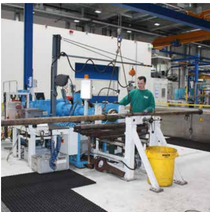
Extruder with stator for oil production
