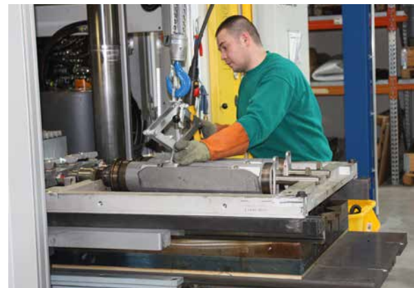
Injection moulding machine for iFD-stators®
