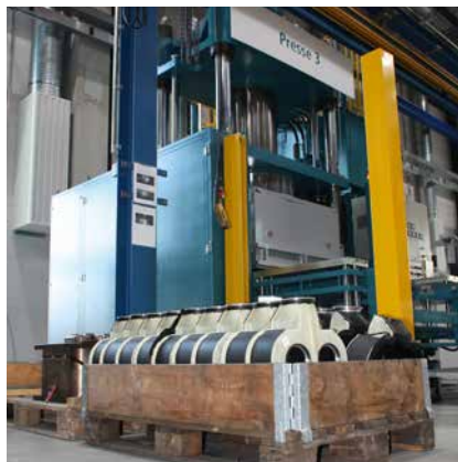
Press with casing liners for TORNADO® T2
