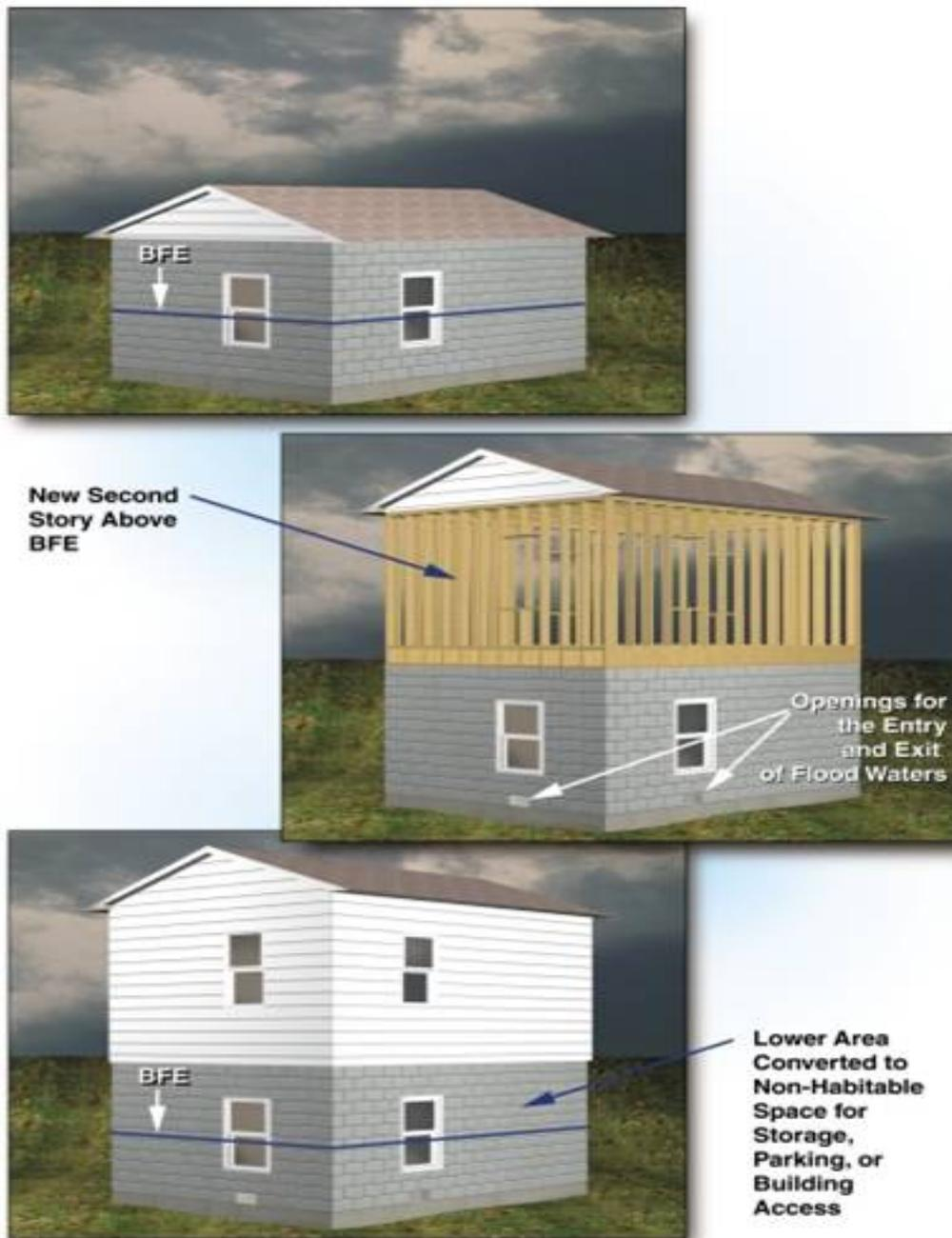
**Figure 5.2: Example of Flood proofing - Raising First Floor of Structure**
