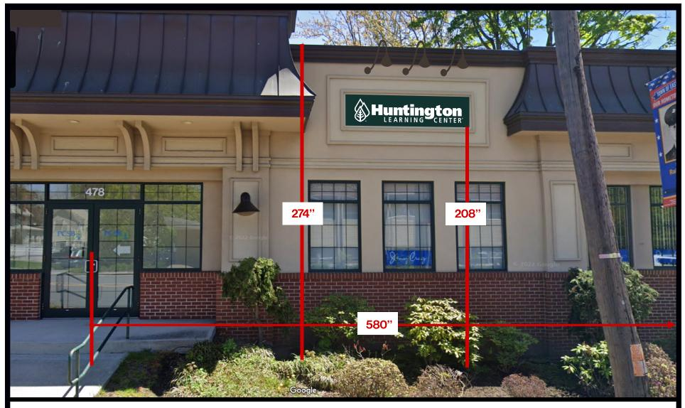
DIMENSIONAL LETTERING ON FLAT BACKGROUND TO MATCH DOOR TRIM - EXTERNALLY ILLUMINATED WITH GOOSENECK LIGHTS
